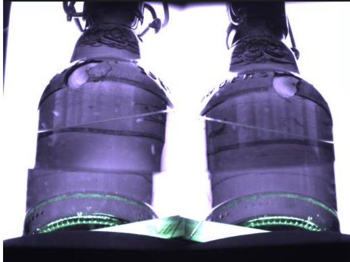
Chipped Shoulder – Detected with optical and X-ray inspection
