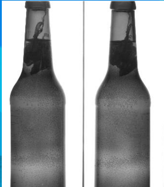
foil in the fill level line
