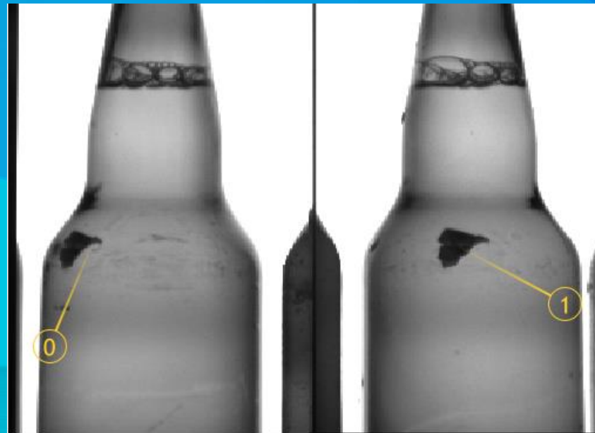
contamination in the shoulder area
