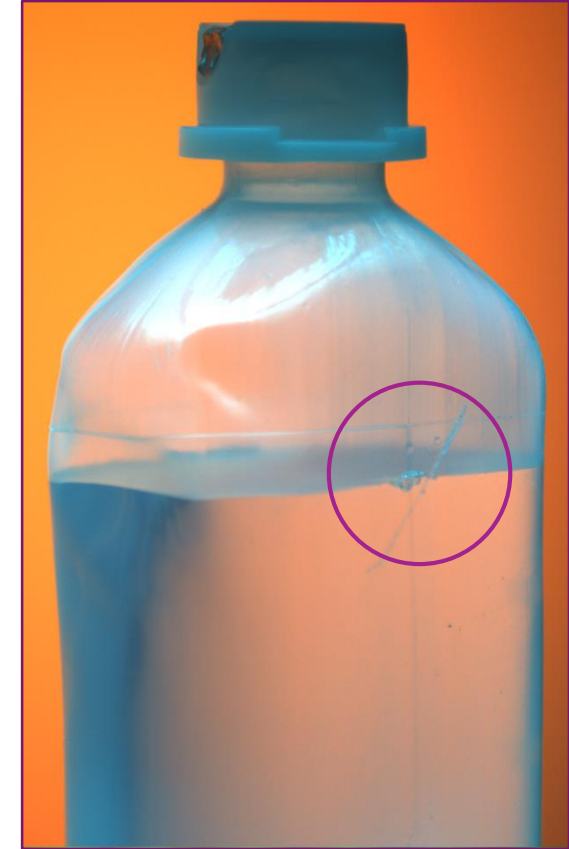
Body damage scratch
