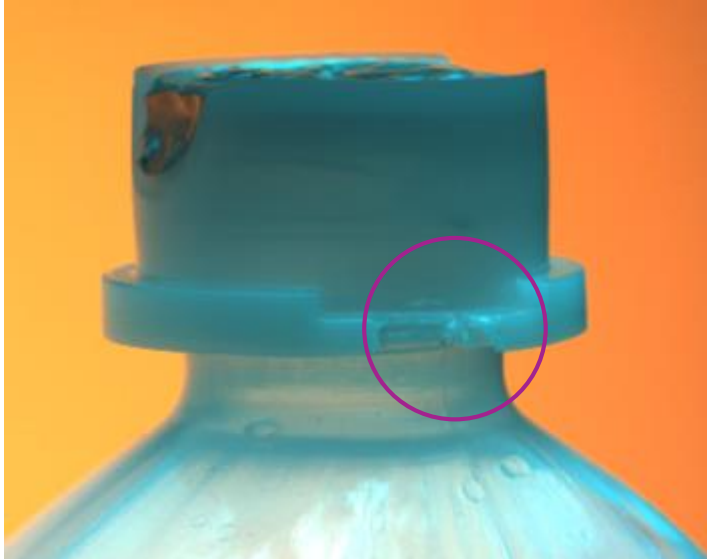
Lack of material sealing ring
