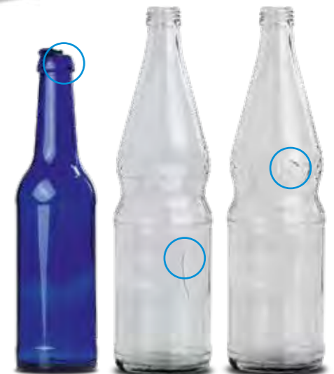
SIMPLY FINDING RELIABLY: finish faults, chips, shell-shaped fractures and many other safety and quality defects.
