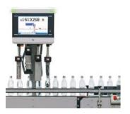
many other quality defects simply reliably. With an integrated quantifying system, serial fault detection and continuous monitoring it uncovers losses in performance of the master machines, such as the filler and closer, before they can bring the productivity of the complete line to a standstill. The "guilty" filler valves and closer heads are located in good time. This makes quality assurance and preventive maintenance simply easy.
