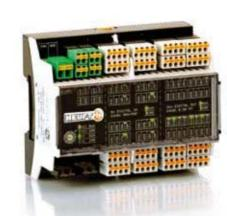
flexibly equipped, networked with each other without any problems and retrofitted at any time. This is even easier now with the new HEUFT ISI real time field bus system - due to the drastically reduced amount of wiring required.
