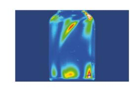
mechanical residual stress which reduces the breaking strength of glass primary packaging visible. Thus the HEUFT InLine IS already identifies critical defects before they can occur. The containers in question are consistently rejected. The HEUFT picCollect collects all the pictures of faults in order to document and archive them sustainably.
