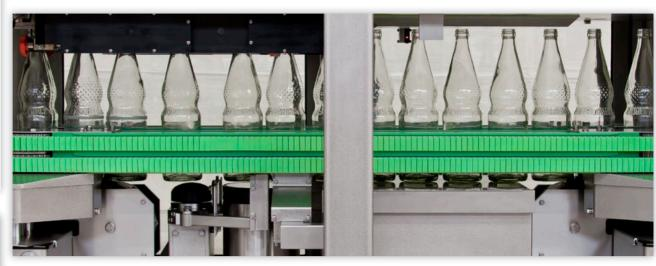
Servo-controlled conveyor belts align the bottles exactly.
