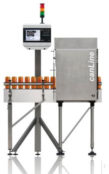
Empty cans which cannot be reliably sealed, are misshapen or contaminated with foreign objects are consistently identified.
