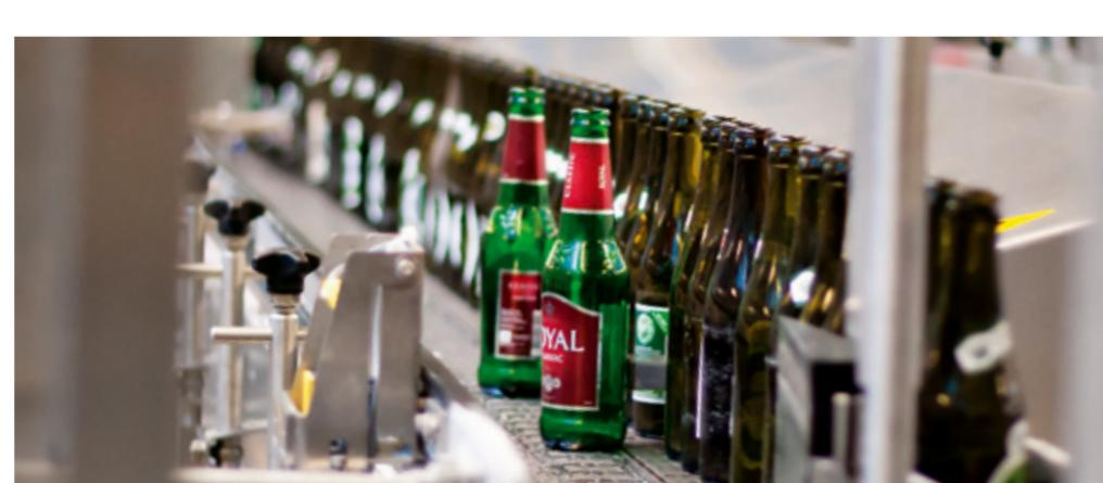
rejection: bottles which are contaminated, incorrectly filled, not sealed or with leaks can each be removed separately from the filling line if required.
